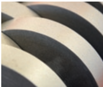
Samicafilm® tapes are thin but show outstanding corona resistance.
